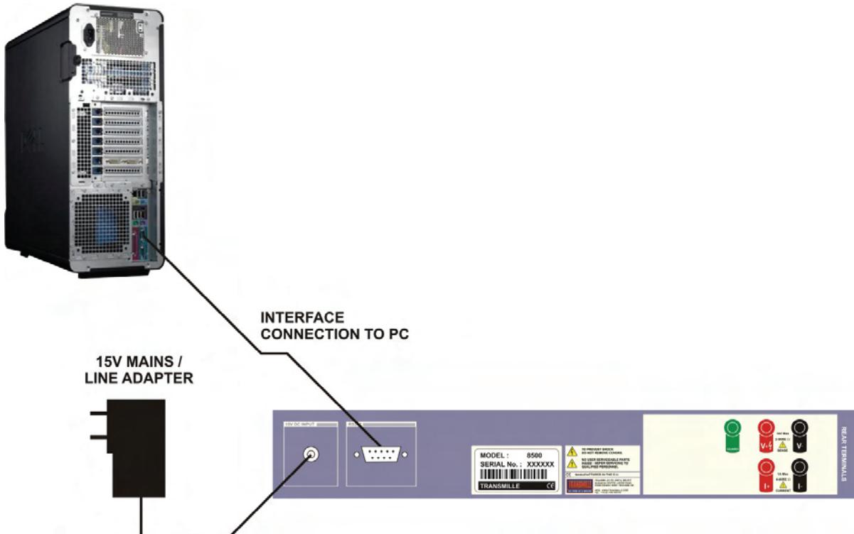
**Connect 15V Power Adapter (supplied) to mains / line and RS232 connection to PC (use RS232 to USB converter if USB connection required).**
