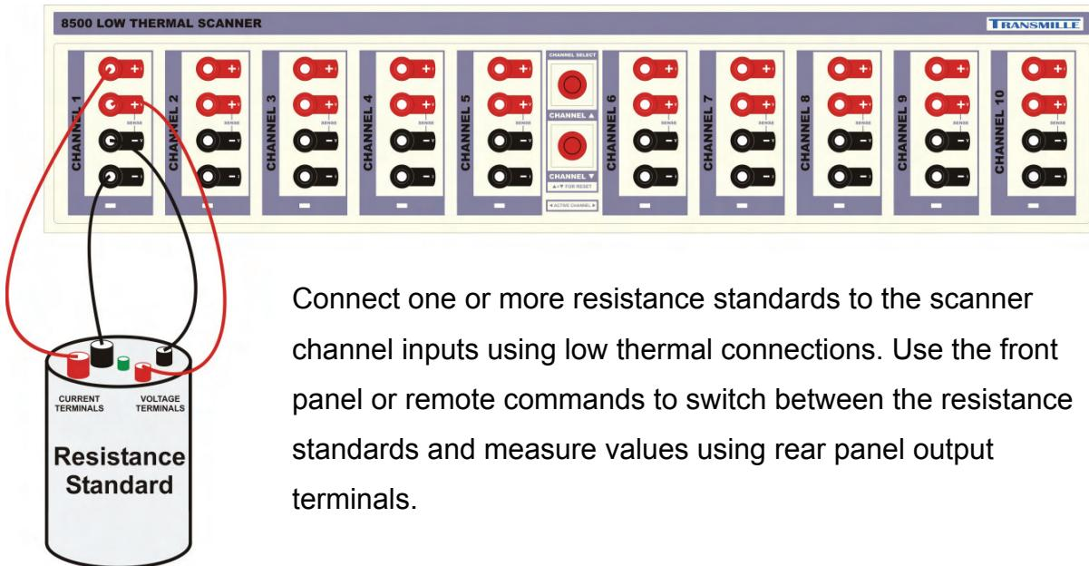
Connect one or more resistance standards to the scanner channel inputs using low thermal connections. Use the front panel or remote commands to switch between the resistance standards and measure values using rear panel output terminals.
