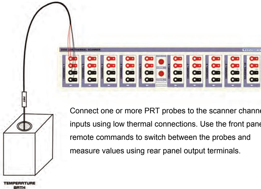
Connect one or more PRT probes to the scanner channel inputs using low thermal connections. Use the front panel or remote commands to switch between the probes and measure values using rear panel output terminals.
